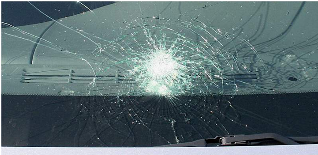
Figure 6: A car windscreen damaged by impact
